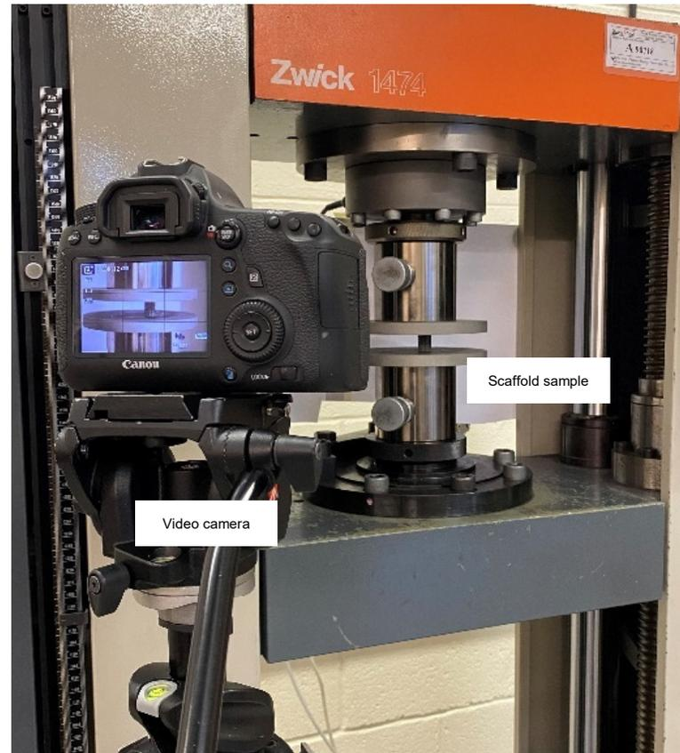
Fig. 8. Mechanical test setup showing compression test for mechanical properties of the auxetic scaffold
